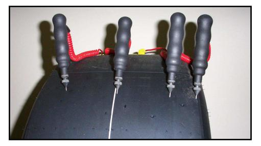
The optimal working range for Goodyear Radial Stock Car tires is from 200 - 250° F. Temperatures higher than 275° F are considered excessive and could lead to tire blistering. This maximum temperature applies not only to the tread, but especially the inside shoulder temperature.
